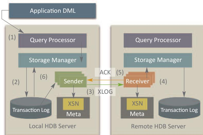
**Figure 2. Synchronous Mode Replication Task Flow.**
