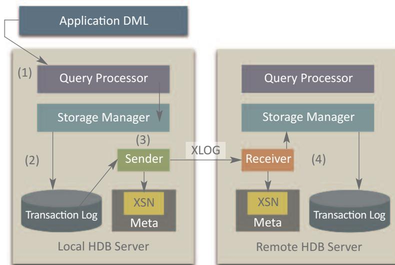
**Figure 1. Asynchronous Mode Replication Task Flow.**
