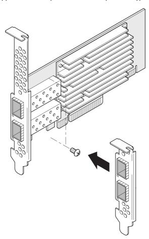
An optional 1PPS bracket and cable assembly, Solarflare part number SOLR-PPS-DP10G, is available for Solarflare dual-port SFP+ server adapters. For detailed fitting instructions, refer to the *Solarflare Server Adapter User Guide*.
